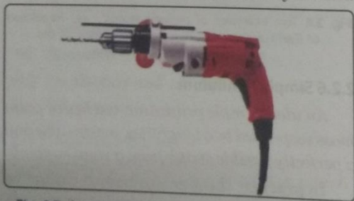
Fig. 2.7 An electric drill. The bit of the drill rotates as well as moves forward into the wood.
